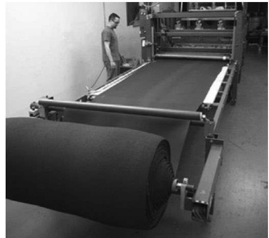
Pressure Sensitive Adhesive Lamination Process
