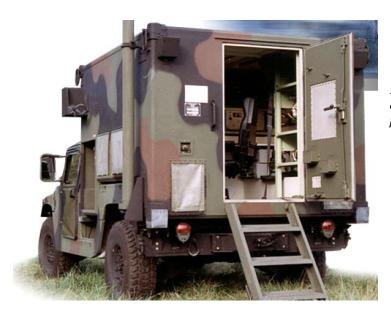
Figure #6 Military shelter utilizing conductive rubber EMI/RFI gasketing on the perimeter of the door.
