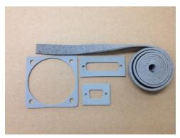
Multicon material is one of the most prevalently used forms of conductive rubber today. It's a combination of silicone and conductive wire paths which provides a superior environmental seal while providing EMI/RFI shielding to frequencies up to 6 GHz.
