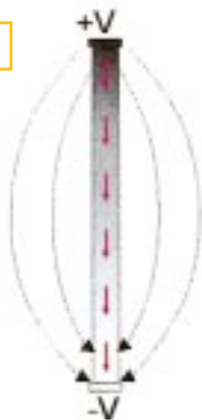
In this depiction of the electric field surrounding a wire carrying a dc current, shades of gray denote the relative voltage levels inside the wire. Magenta arrows denote the current.
