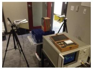
Figure #2 Radiated testing of MAJRabsorber
